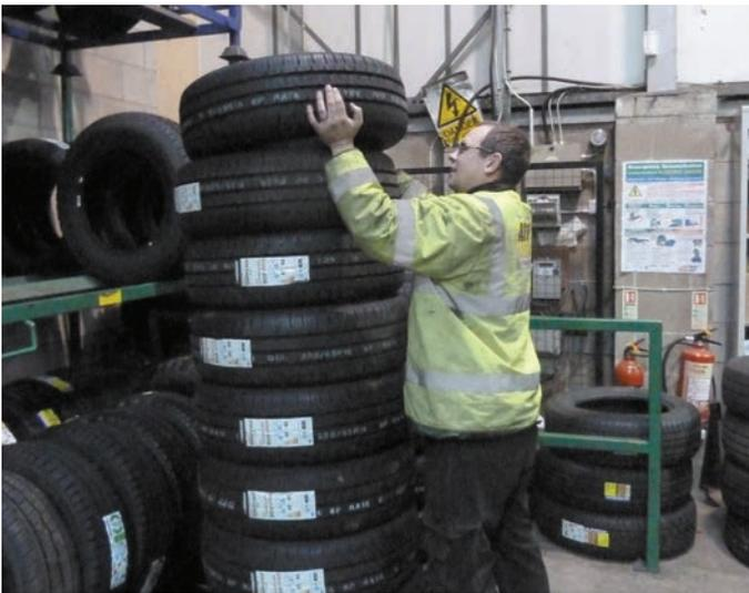
Lifting of tyres to and from a high location is awkward and potentially hazardous. Stretching to reach the top of the stack creates a posture with an increased risk of injury. Also, high stacks may collapse onto people. The weight of a high stack can damage the walls of tyres at the bottom. Manually handling tyres of over 10kg in weight onto high stacks creates the following risks:
